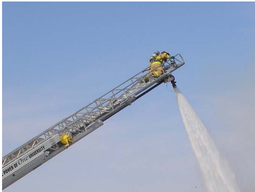
An NMSU Firefighter uses an aerial mounted master stream to extinguish a large commercial vehicle fire.
